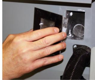
1. Pull the Debris Separator out of its holder on the printer.
