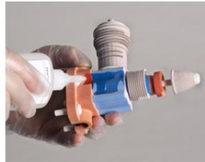
1. Drizzle Z-Bond onto the part. Start with the most delicate areas first. Wet as much of the part as you can easily reach.
