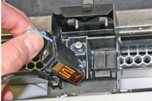
3. Open the printer top cover. Open the carriage cover and lift the print head out of its slot. Properly recycle or dispose of the empty cartridge.
