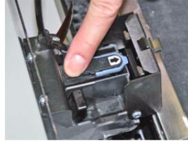
7. Insert the new printhead. Press down firmly on the top of the printhead, on the same side as the pogo pins, to securely fit the printhead into its slot.
